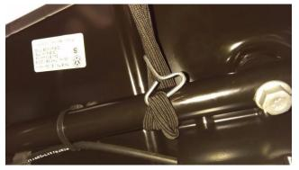
Pop the bottom cover into position – feed the rear through the spilt in the rear of the seat and the bungee cord down the sides of the plastic covers, feeding through to the rear as pictured below.
