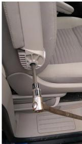
Next remove the plastic cover on the arm rest, taking care not to scratch anything. Using the M10 Spline tool remove the bolt from the armrest. Be sure to use socket wrench so you put pressure onto the head of the bolt, some customers have used ring spanners on the shaft of the spline too and as a result stripped the head of the bolt.
