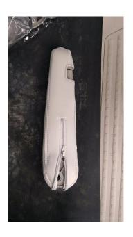
Feed the armrest covers on (use some silicone lubricant spray or dashboard shine spray and lightly spray inside the cover if this proves difficult to fit.
