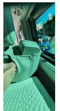
Using the two areas below to pull, begin drawing the zips down, working a couple of inch one side then a couple of inch on the other side, please do not use the zips to pull the cover together – this will break the zips.
