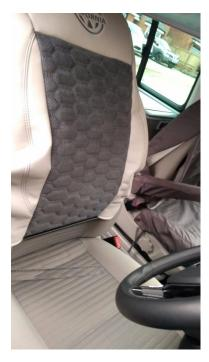
Remove the headrest and Slide the back rest cover over the seat and into position. The Cuts on the top of the cover fit over and under the head rest posts.
